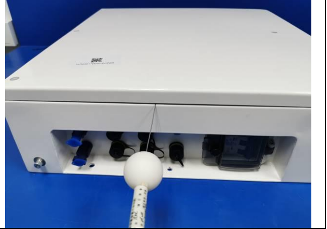
No.4-2 IP6X test (Protection against access to hazardous parts)
