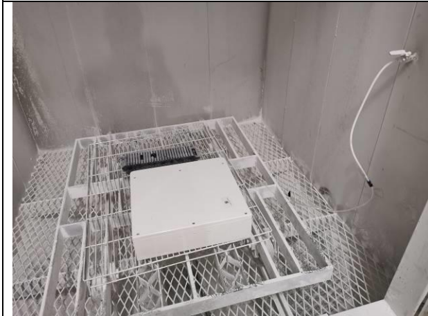
No.4-3 IP6X test (Protection against solid foreign objects)
